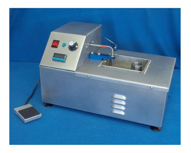
Wave soldering pot, to use lead-free solder, a recent design, intended for intensive use in industry.
